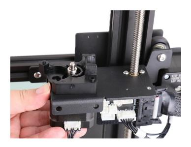
4. Place the white gear assembly into the groove near the stepper motor gear and align them well.
