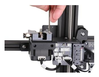
2. Install the provided gear onto the motor shaft with the set screw side up and tighten the set screw. Note: make sure the gear section is underneath and set screw is on the top when install the new gear.
