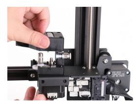
7. Insert the bolt with a spring and a washer into the puller hole and screw it a little tight.
