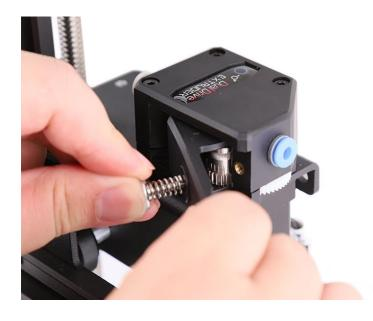
8. Insert the Bowden tube into the coupler as deep as possible and then clip it tight.
