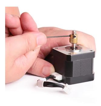
3. Put the motor back into the mount. Place the bottom half of the extruder on to check the gear alignment and adjust it if needs to.
