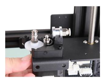
6. Put the top part of the extruder on and then secure it tight. Perfectly align gear parts and then assemble the top parts of the extruder on.
