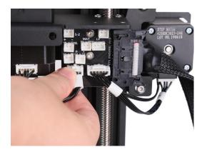
Tips: motor direction will be reversed and we need either change it in the firmware or invert motor cable wires.
