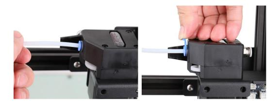
9. Plug in stepper motor wiring and other wires on the circuit board. Cut the PTFE tube into appropriate length for your 3D printer, and then insert it into the other coupler on the other end of the extruder and clip it tight.
